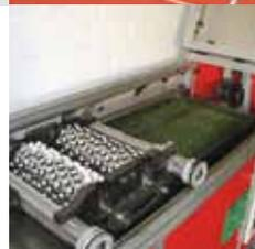
*Wear resistance test for artificial turf*
